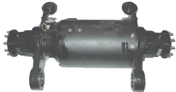
Heavy duty drive axle (The drive motor is coaxial with drive axle) with internal wet disc brake.
