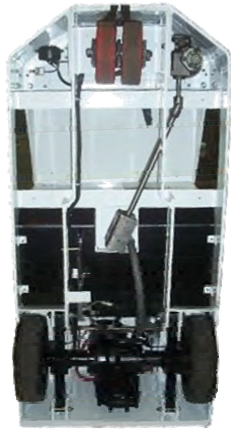
Under side of Frame Shows the one-piece welded frame, as well as the strength of the frame due to the inner frame rails.
