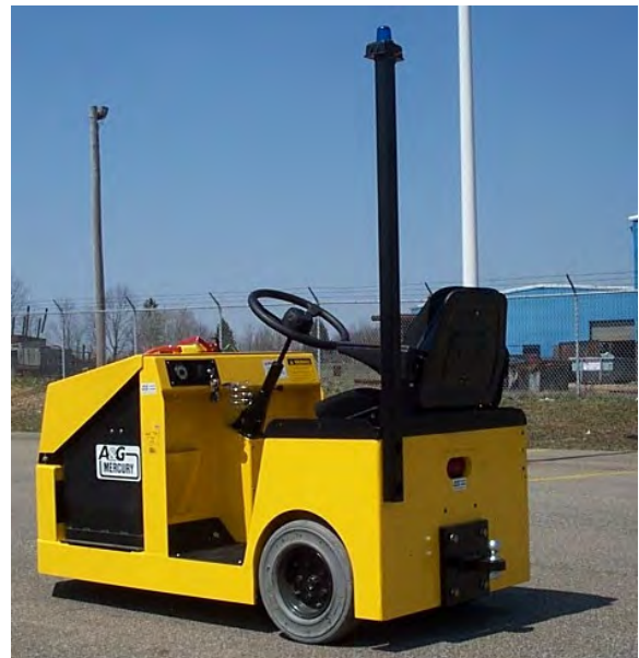
Note: Shown with Optional Strobe, Quick Charge Battery Connectors, & Rear Ball Hitch.
